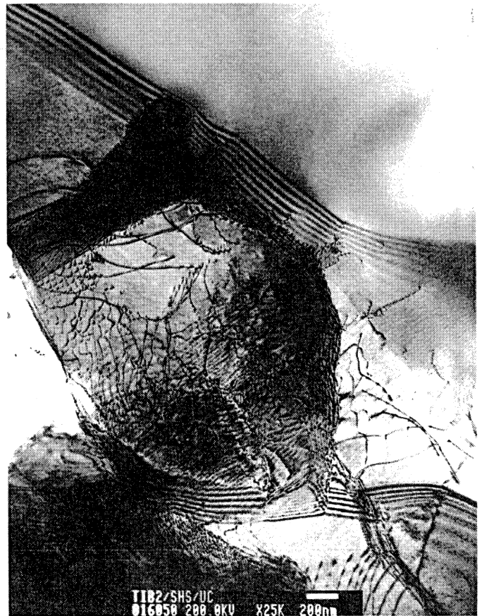
Figure 10. Transmission electron micrograph of \text{TiB}_2 showing grain with dislocations.
